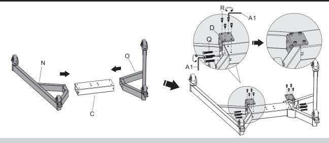
Insert the right base into the base. Align the holes on the right base to the holes on the base .Fix the base with the connecting plate and the screws. Repeat this step for the left base.
