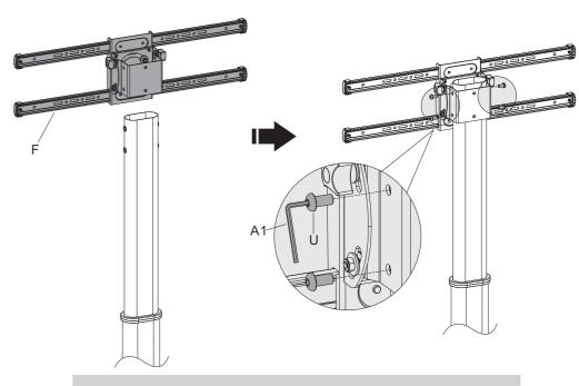
Attach the universal plate to the column using the appropriate screws.
