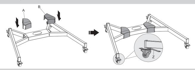
**NOTE:** Lock the brakes on the casters to avoid any unexpected movements during installation.
