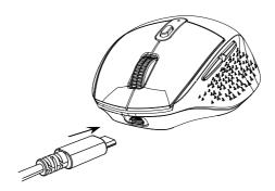
While charging, power light turns red. It needs 4-6 hours to be fully charged. The red indicator light will turn off after fully charged. Also, when the battery power is too low (around 3.2V), the red light will flash to remind charging the mouse.
